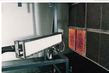
B) Test start on MDF coated with the TB cycle.
